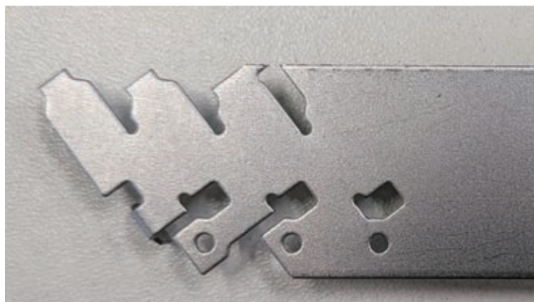
図5 プレス工程サンプル Progressive forming sample in several operations
